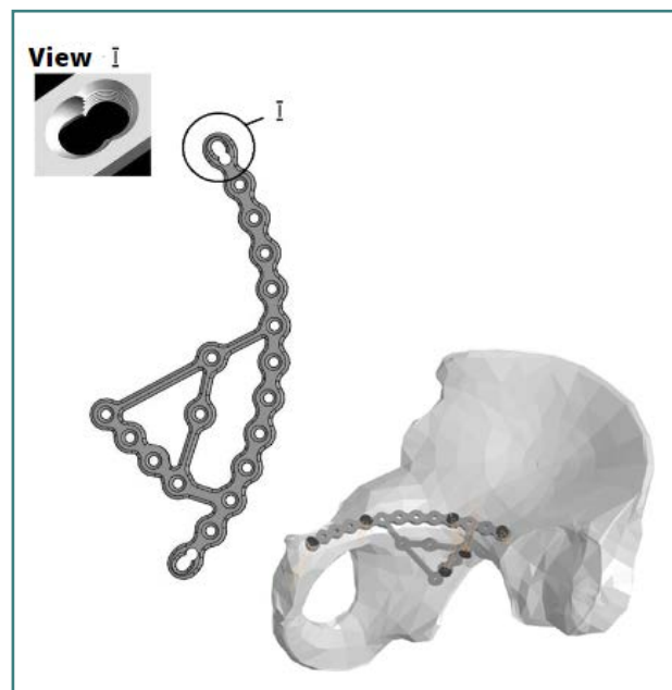
Figure 2. Orthopedic plate visualization (A) and pelvic system 3D model (B)
