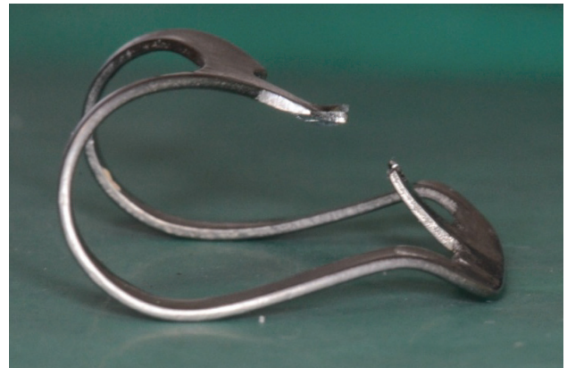
Fig. 6 Clamp 212 modified by changing the jaws' orientation (method described in the specific literature [1,2]).
