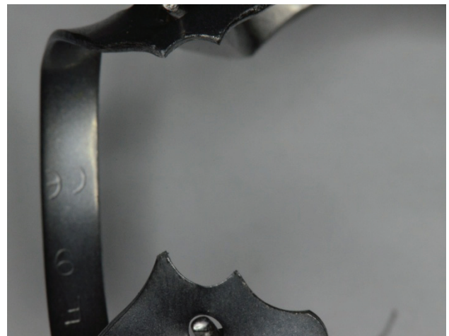
Fig. 33 Clamp no. 1 modified: active contour and contact points
