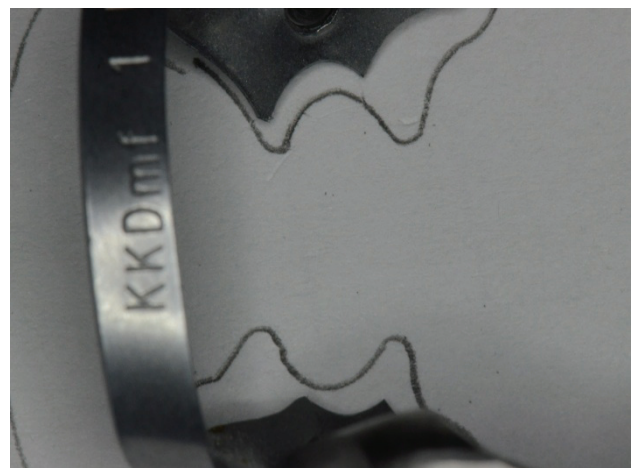
Fig. 34 Notice the difference between the initial contour of the standard clamp (drawn on the paper) and the modified one, according to the real contact section
