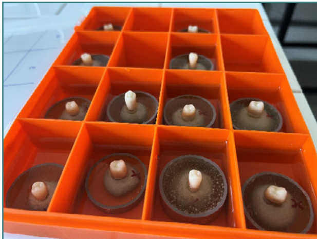
Figure 8. Macroscopic view of a tooth embedded in the support structure used for mechanical testing
