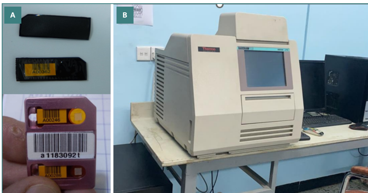
Figure 2. Thermoluminescent dosimeter (TLD) and reader setup for dose measurement. A, TLD encapsulated in a disposable vinyl pouch 7mm/cm 2 . B, TLD Reader, Harshaw Model 6600; Harshaw Thermo Fisher Scientific
