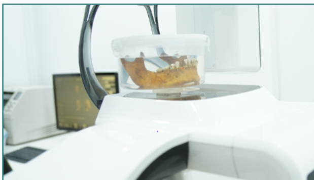
Figure 3. Dry mandible immersed in water for image quality assessment
